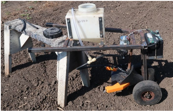
Photo 3. One-row 360 Y-DROP® applicator for application of V14 fertilizer treatments in small plots at Lamberton, MN and Waseca, MN.
